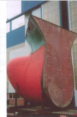
Forepeak, ready to be installed
