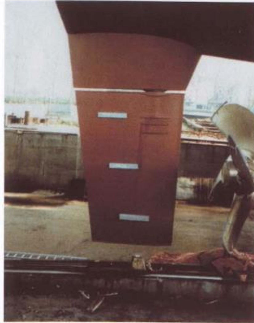
A spade rudder on a reefer, freely suspended from the rudder dome
