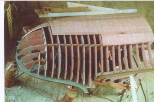
Fitting of the shell plating
