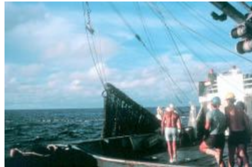
Securing rings to the ring stripper prior to net retrieval (Figure 4 in Itano 2003)
