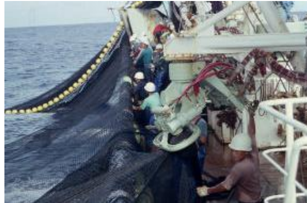
Sacking up with rail roller and pinch hauler on Japanese group seiner (Figure 23 in Itano 2003)
