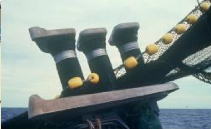
Triplex power block (Gillett) (Figure 14 in Itano 2003)
