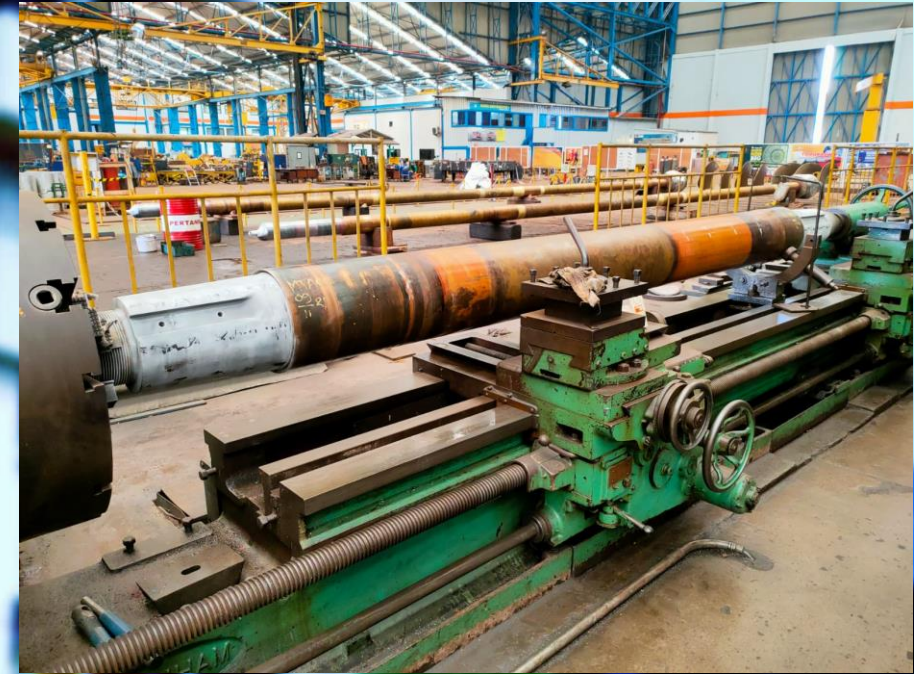
(Pengecekan keretakan shaft by PT )
