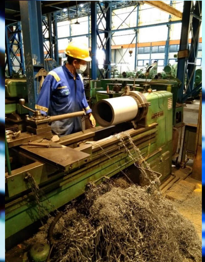
(Machining bantalan baru)
