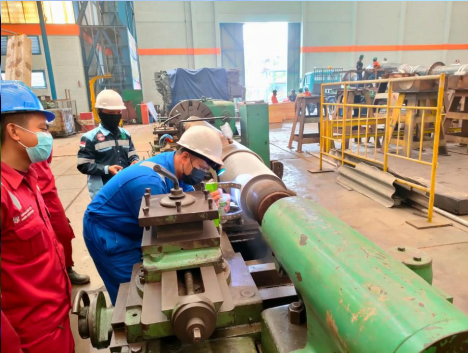
(Pengecekan keretakan shaft by MPI )
